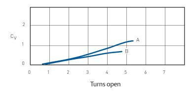
A =  $\frac{1}{4}$  inch (6.4 mm) orifice, valve  $C_V$  1.4 maximum B =  $\frac{3}{16}$  inch (4.8 mm) orifice, valve  $C_V$  .83 maximum
